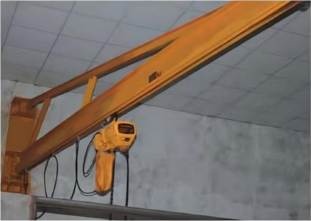
悬臂吊 Jib Crane
